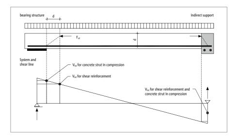
Single loads near direct support (0.5d  $\le$  a<sub>v</sub> < 2d) may be decreased by the factor  $\beta_E$  for shear design.
