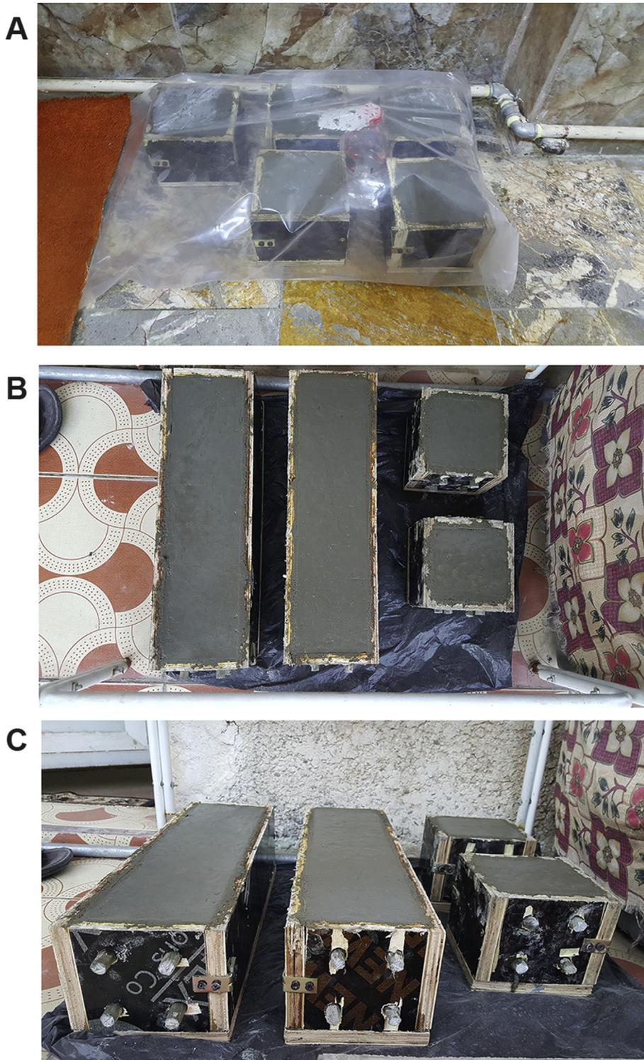
Fig. 3. (A–C): Casting of specimens.
