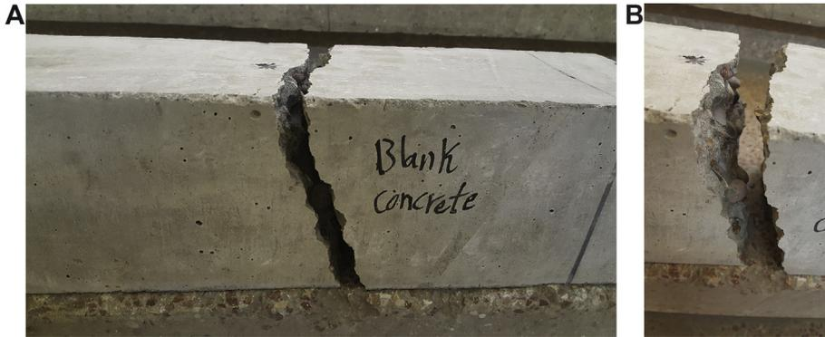
Fig. 8. (A, B): typical fracture of unreinforced concrete.
