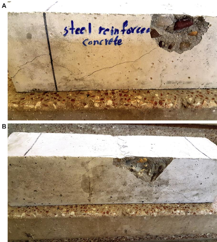
Fig. 11. (A, B): typical fracture of steel RC.
