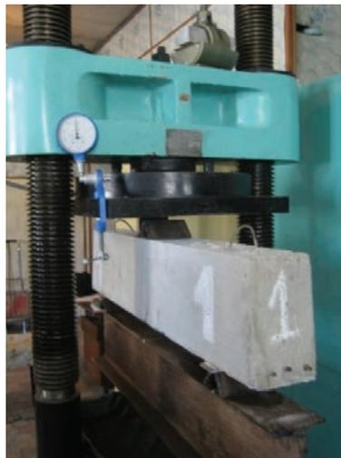
Fig. 1. General view of the test rig beams bending
